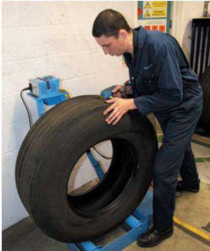
Figure 2. Manual tire regrooving
