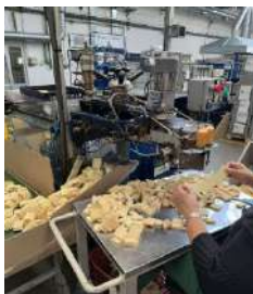
Figure 2. The industrial stapler for joining ends of the paper filter
