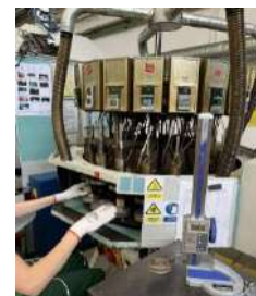
Figure 5. Circular press for pressing and sealing filters
