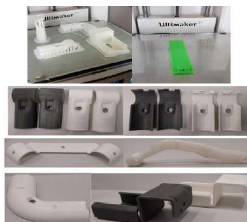
Figure 10. Scanned elements made with 3D printing technology
