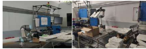
Figure 18. Process of stacking and packing bags using a collaborative robot in experimental conditions inside the Learning Factory at the Faculty
